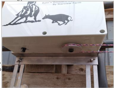
If the knob is turned all the way down, the flag may not move at all. Adjust this from the ground before starting work.
