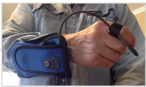
on either their index or 2<sup>nd</sup> finger, with their finger tip above or near the 'boost' button on the end of the finger control. The direction switch is spring loaded and is actuated with your thumb. The system is designed to keep your hands free to hold reins.
