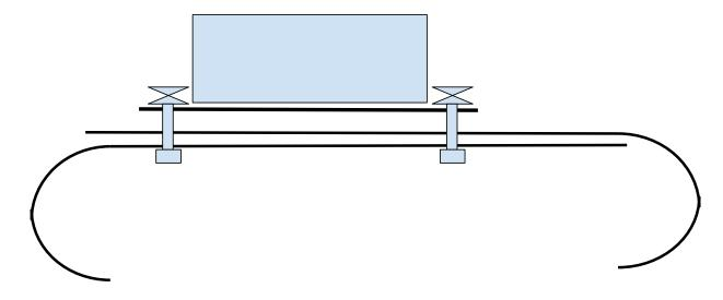
When assembled, lift and turn the unit upright. Mount the top slide onto the top rail of your fence. Slide the system towards a vertical rail of the fence, or add a blocker board, so the tension of the line will pull the unit against a rail. This keeps the unit from sliding towards the idler.
